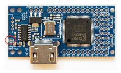
Then power the board with 5V (UNREG pin) and the HDMI DDC line will be powered through the resistor. Do not use a voltage higher than 5V to stay compatible with HDMI.
